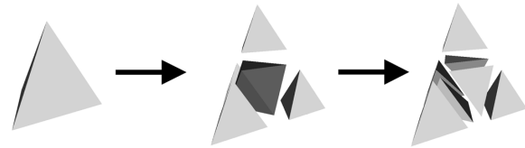
Figure 2: Splitting a tetrahedra generates an octahedron in the middle. Splitting the octahedron into tetrahedra requires the choice of a diagonal.
